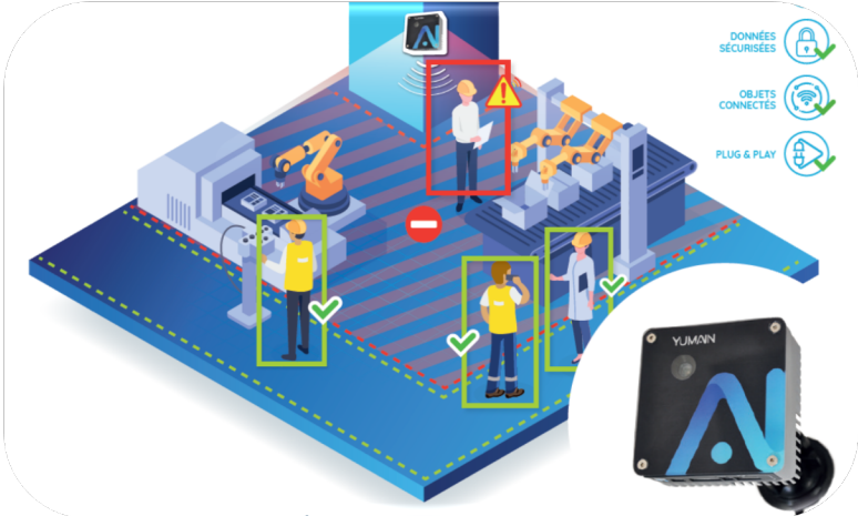
Image 1: The Yumain sensor monitors an area in a machine hall in which workers are allowed to move (green) or are not allowed to move (red). The sensor registers when workers step in the restricted area and gives a signal or stops the machine.
