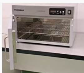
Chamber for physical disinfection of filtering half masks - UV-C radiation
