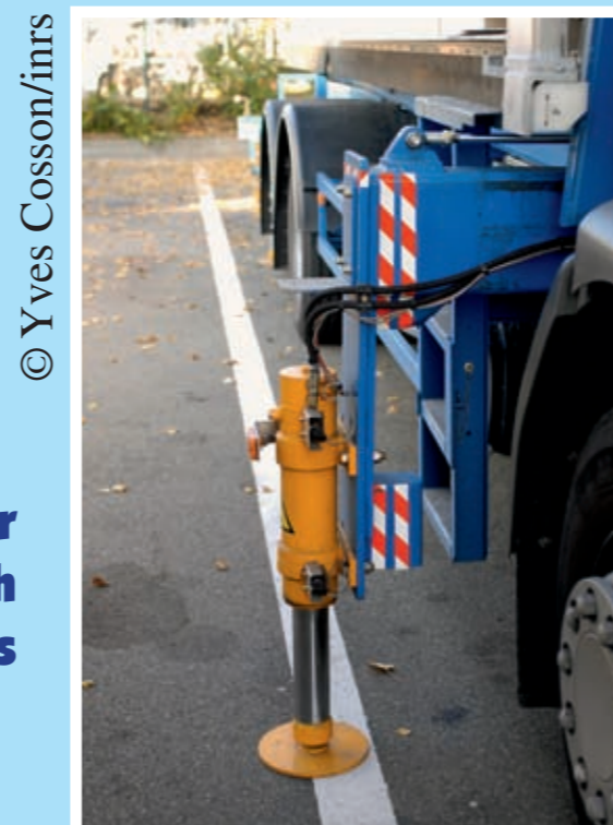
Stabilizer with interlocks
